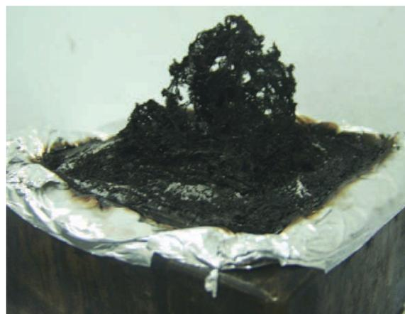
Figure 13 Picture of char residue under cone calorimeter testing of PC. [Color figure can be viewed in the online issue, which is available at wileyonlinelibrary.com.]
