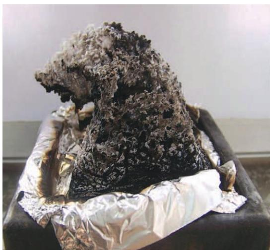
**Figure 14** Picture of char residue under cone calorimeter testing of PC/6 wt % OPS composite. [Color figure can be viewed in the online issue, which is available at [wileyonlinelibrary.com](http://wileyonlinelibrary.com).]
